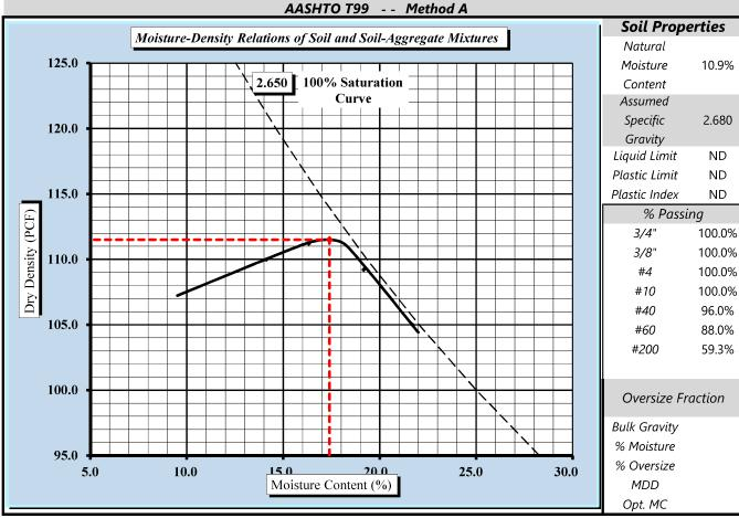
Corrected for Oversize Fraction (ASTM D 4718) Moisture-Density Curve Displayed: Fine Fraction 🗵 Sieve Size used to separate the Oversize Fraction: #4 Sieve 区 3/8 inch Sieve □ 3/4 inch Sieve □ Mechanical Rammer Manual Rammer ⊠ Moist Preparation □ Dry Preparation ⊠
